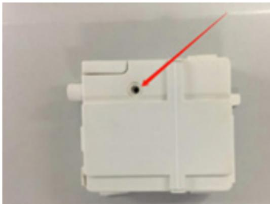
1.3 Insert WiFi module as shown in the figure (The "Smart kit" is marked face up)
